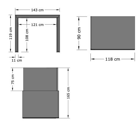
The integrated sound absorber frame is filled with 17 mm A-classed sound absorbing material on both sides of a 8 mm solid wooden board. Hilo is coated with a 3 mm foam laminated fabric.
