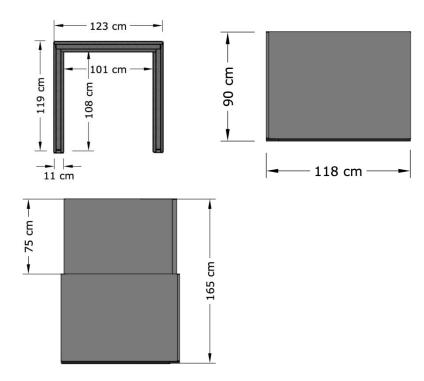
The integrated sound absorber frame is filled with 20 mm A-classed sound absorbing material on both sides of a 6 mm solid wooden board. Hilo is coated with a 3 mm foam laminated fabric.
