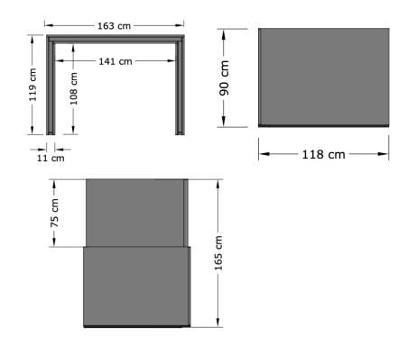
The integrated sound absorber frame is filled with 20 mm A-classed sound absorbing material on both sides of a 6 mm solid wooden board. Hilo is coated with a 3 mm foam laminated fabric.
