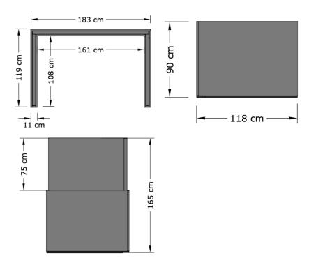
The integrated sound absorber frame is filled with 20 mm A-classed sound absorbing material on both sides of a 6 mm solid wooden board. Hilo is coated with a 3 mm foam laminated fabric.
